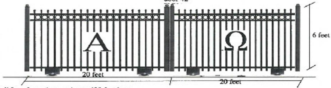
\* Furnish and install Iron fence ( approximate 630 feet long and 6feet high. pickets 3/4 X 3/4 X 16 gauge. posts 3" X 3" X 14 gauge X 6' high. with Black Metal Fence Mounting Bracket.
